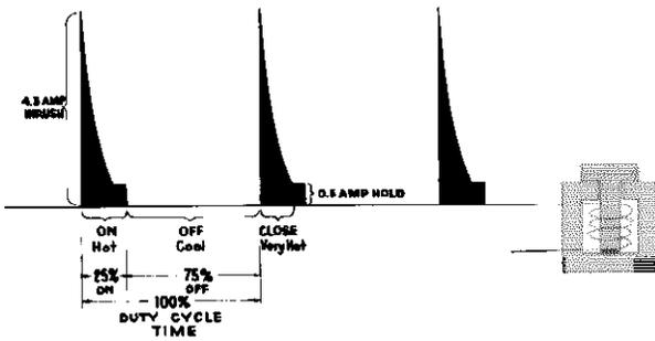
Each time the solenoid is cycled it receives a pulse of high inrush current which gradually declines as the plunger closes. In the full closed position, the solenoid is held energized by a low holding current flowing through the coil until the solenoid is de-energized.
