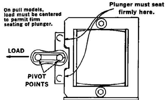
5. Solenoid force drops when line voltage drops. Always select a solenoid large enough to move the load at the minimum design voltage. Decco graphs show solenoid force at 100% and 85% of rated voltage.
