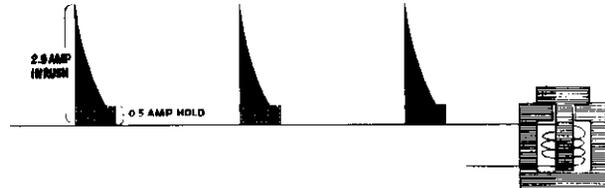
We also know that a solenoid's speed of closing is dependent upon the load it must move. If we reduce that load, we further reduce the heat generating area and our chart looks like this:
