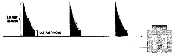
The shaded area represents the reduction in closing time (area of heating) affected by lightening the solenoid's load.
