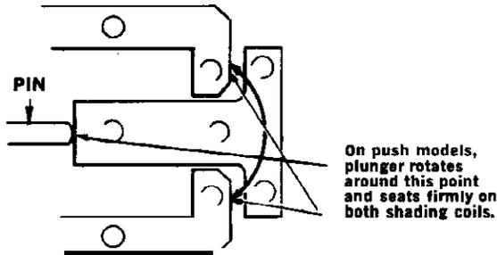
2. Use the shortest possible stroke to reduce impact force and solenoid wear.
